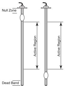
If Level or Interface Float are outside of active region: **Analog Mode** 3.7 mA
