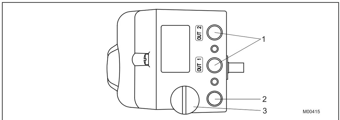
Fig. 18: Pneumatic connections
